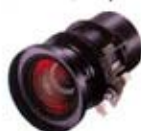
Option 1 FS501 (Short fixed) Lens shift position 1:1, F=2.3, f=16mm, Throw distance ratio = 0.8:1, zoom: 1.0
